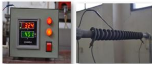
Figure 6 Heating coil and temperature measurement.
